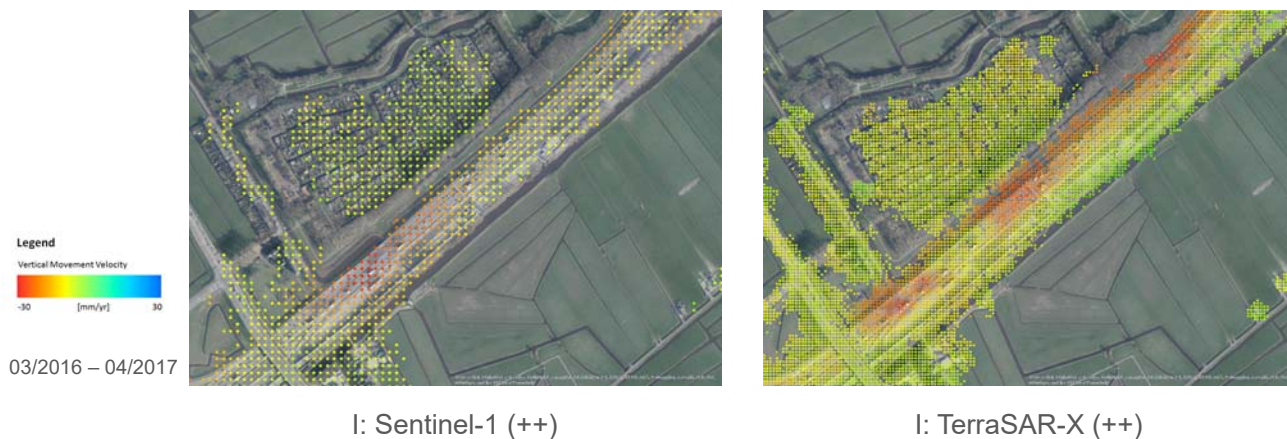
Subsidence of recent built traffic lane
